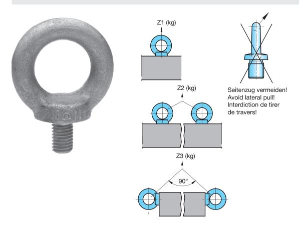
Ring bolts according to this norm serve principally as load carrying device for the lasting fixing of components like engines, electrical cabinets, gears and so on, for their transport. Ring bolts with the next larger diameter have to be used for the alternating use with different articles which have to be transported, like for example big tools. Concerning the utilization of multiple strings slinging means, the rules, for example, according to DIN EN 818-4, have to be considered.
