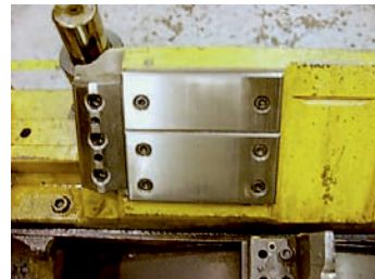
■ SNS-sintered metal and counter bearings after 187.000 strokes
