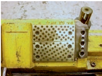
■ With solid lubricant and counter bearings after 187.000 strokes
