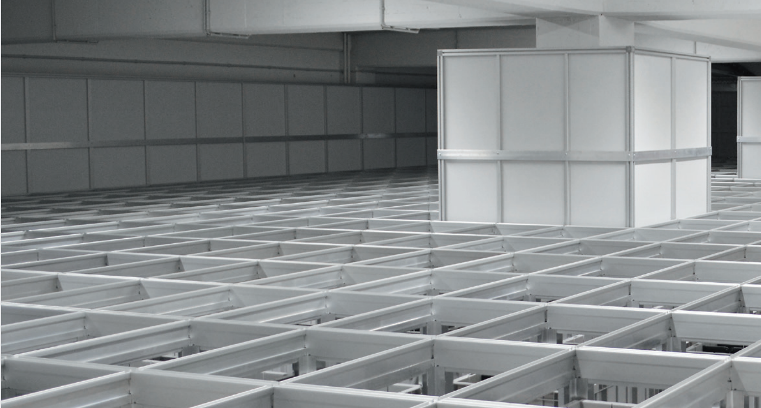
Compact storage on 14.000 storage sites operated by 4 robots.
