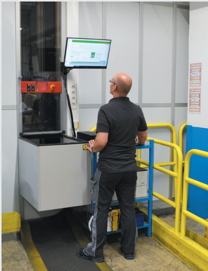
Intelligent storage system with 8.500 containers stacked on the top of each other.
