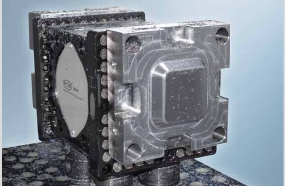
The elements of the BreyLine construction kit of FCS systems allow a five-side machining poor of interfering contours.
