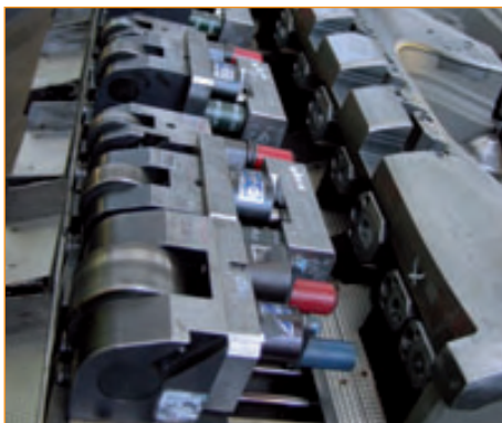
■ More than 30 roller cams SN 5620 are in action for the die-cutting of the holes in the deep-drawn side-panel.
