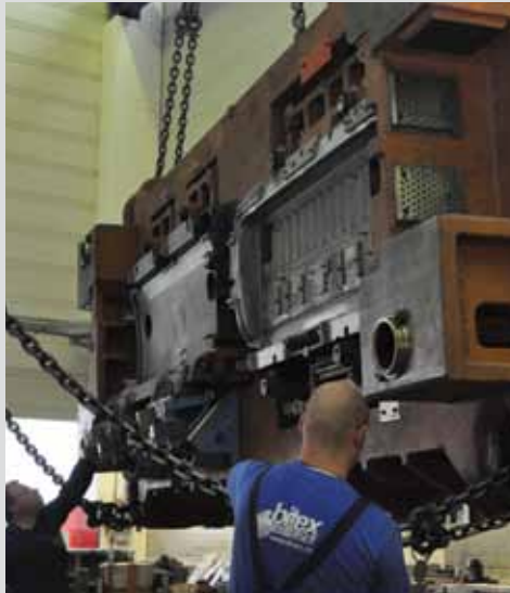
Employee of Schwarz when turning an upper part of a tool which has a length of 5 meters
