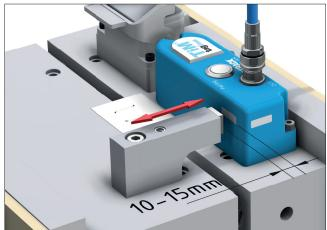
TiM has two proximity sensors mounted on the side of the housing which allow to count cycles. For this purpose, a magnet SN10170 is approximated within 15-10 mm to the sensor surfaces to trigger a counting cycle. The sensor surfaces are marked with white areas on the housing. Furthermore, external signals can be processed via sensor inputs to mount TiM for example at a more remoted location and however be able to register count cycles of the tool.
