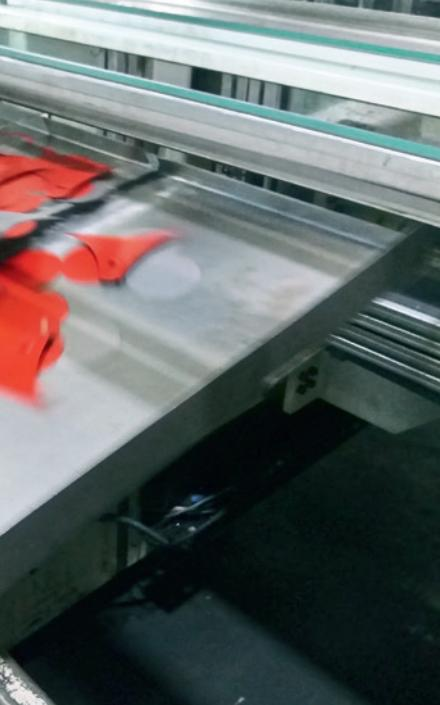
The linear conveyors operate according to the principle of speed difference due to different surface friction values. There, different front- and back acceleration values are used to transport parts or punching waste on a sheet groove.
