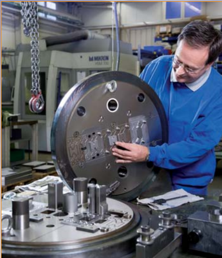
STRACK NORMA delivers the precision die sets for the complex tools of the company SODECIA
